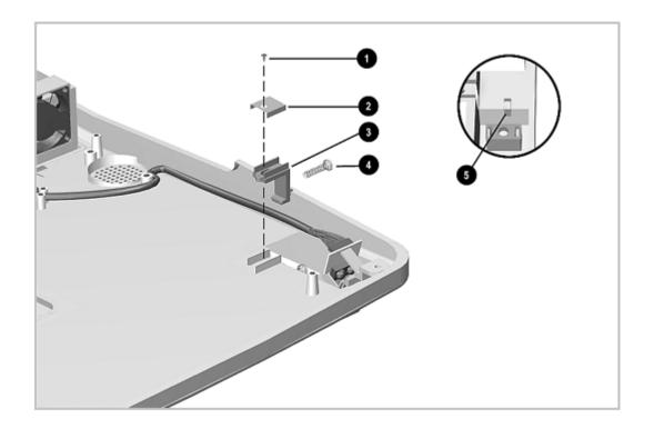
Figure 7-32. Removing the CPU Guide
